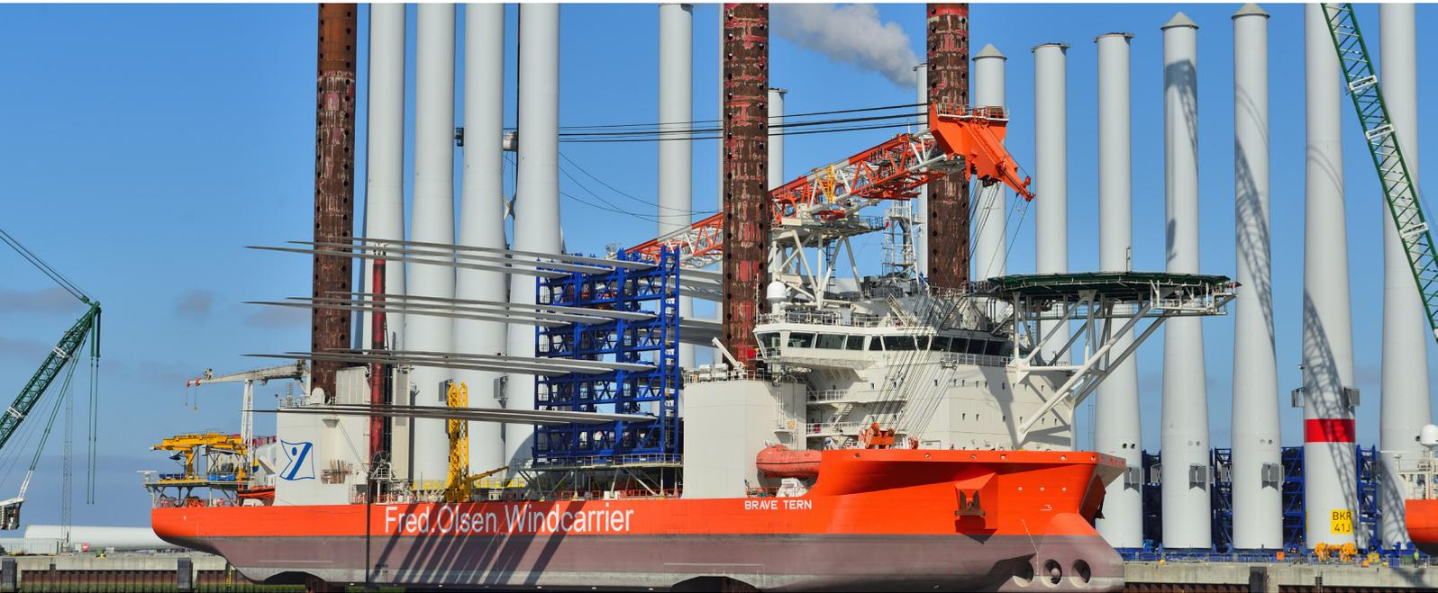
On 20 January 2019, Fred. Olsen Windcarrier's jack-up installation vessel Brave Tern successfully installed the final turbine, completing the installation of MHI Vestas turbines on Horns Rev 3.
