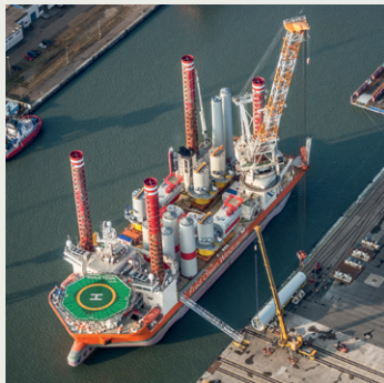
Bold Tern loaded with towers and nacelles copyright: Global Tech I / Henthorn
