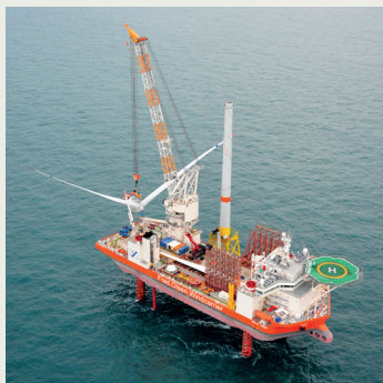
Bold Tern lifting the nacelle from its deck
