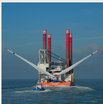
Bold Tern under way with the 6MW Haliade 150 turbine
